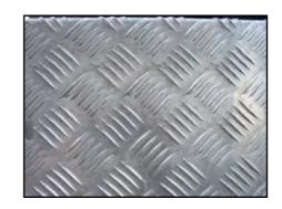
Metals also have a characteristic of malleability. Malleability is the ability for metals to be hammered, pressed, or rolled into thin sheets. The figure shows a piece of metal hammered and pressed into a piece of sheet metal.
